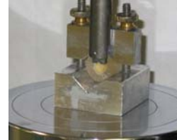
Figure 2: Shear Bond Test Set-Up
